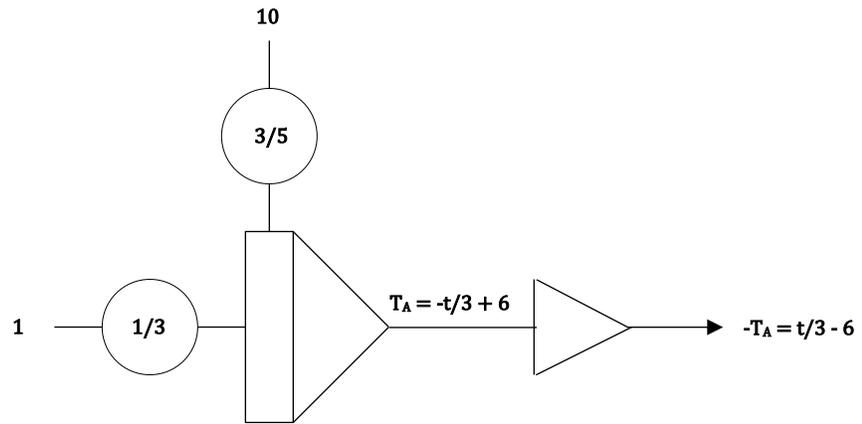
Figure 1: Computer setup to generate decreasing ambient temperature
