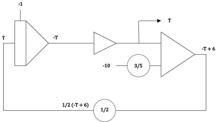
Figure 1: Computer setup for Newton's Law of Heating Simulation ( $T_A = \text{constant}$ )
