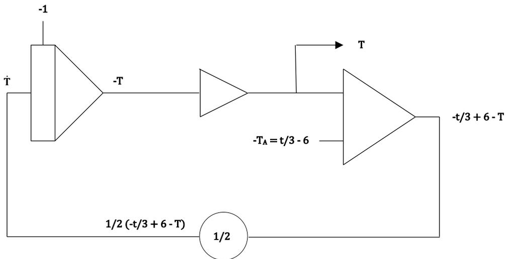
Figure 2: Computer setup for Newton's Law of Heating Simulation
