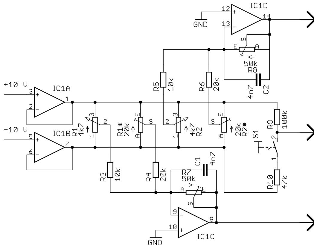
Figure 1: Joystick adapter circuit
