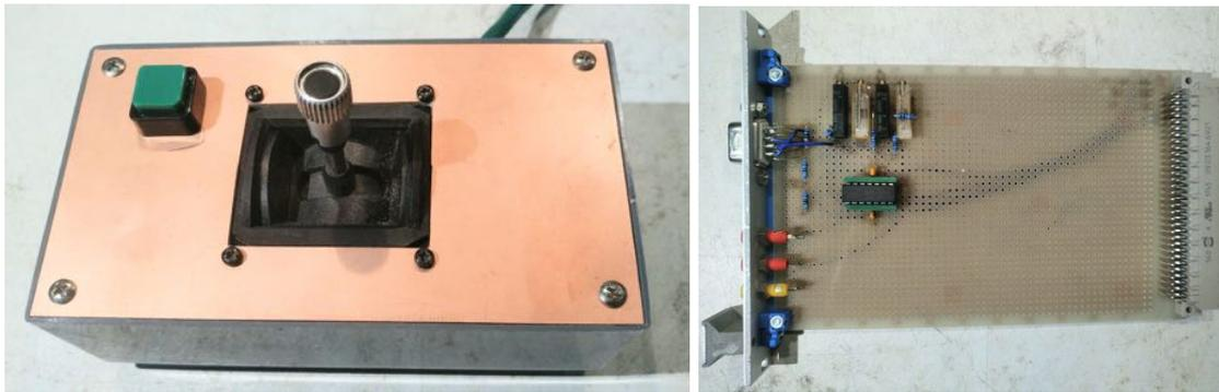
Figure 2: Joystick mounted in enclosure and prototype adapter circuit
